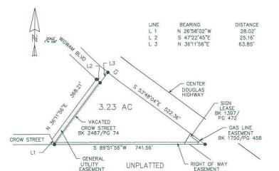
CURVE DELTA ANGLE RADIUS ARC TANGENT CHORD CHORD BEARING 02'48'26" 1532.39' 75.08 37.55 75.07 S 51'51'59"E
